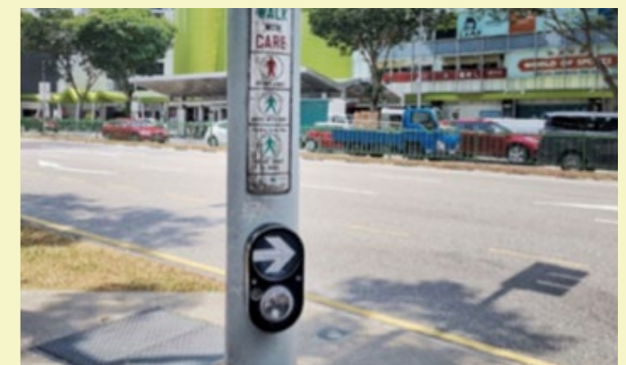
Figure 3. Singapore – Green Man plus at pedestrian crossings
